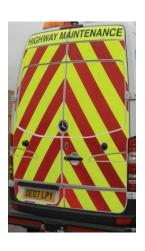
Chapter 8 requires high visibility rear vehicle chevron marking for vehicles stopping on the highway for works purposes or inspections. O5.2.3(c) states; Chevron markings comprising alternate strips of retroreflective red material and fluorescent yellow non-retroreflective material, of not less than 150mm width each, inclined at 45-60° to the horizontal and pointing upwards, should cover as much of the rear-facing portion of the vehicle as possible ... "
